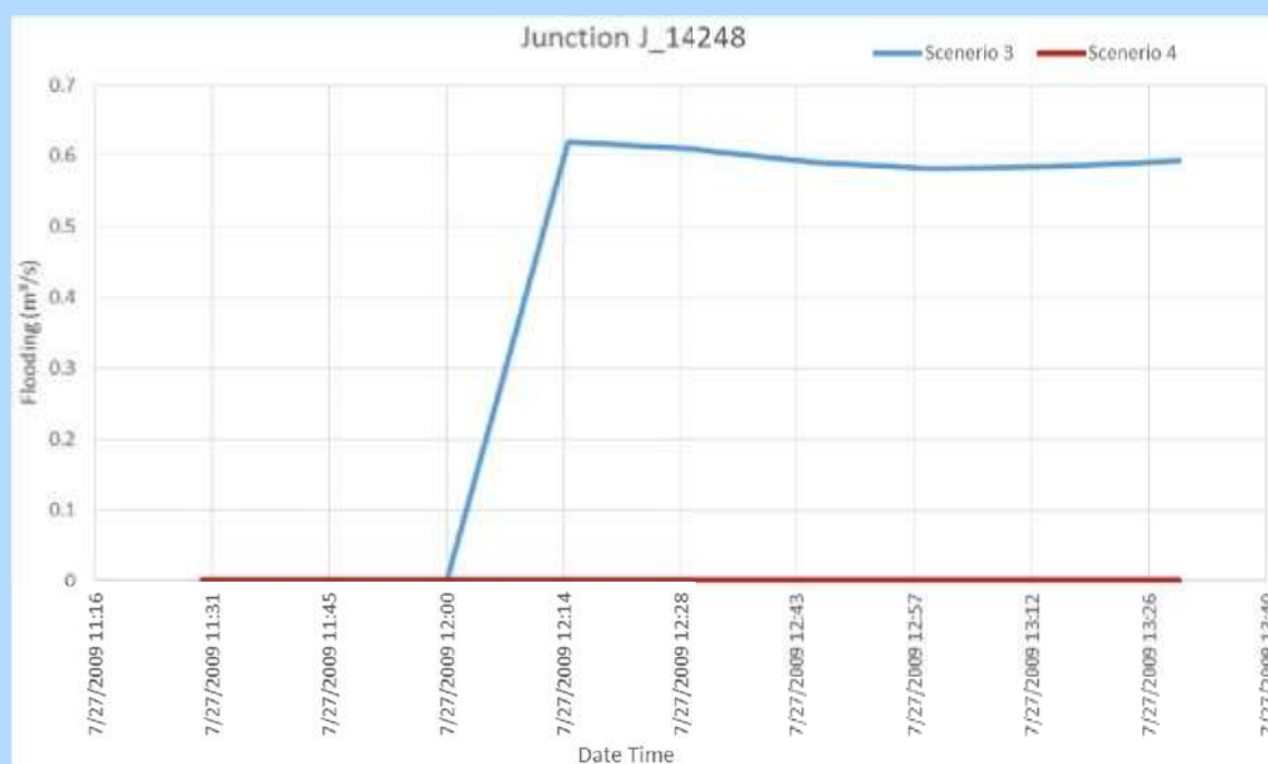
Figure 3.2-19: Comparison between the flood volume at a sample junction after simulation of scenario 3 and scenario 4
