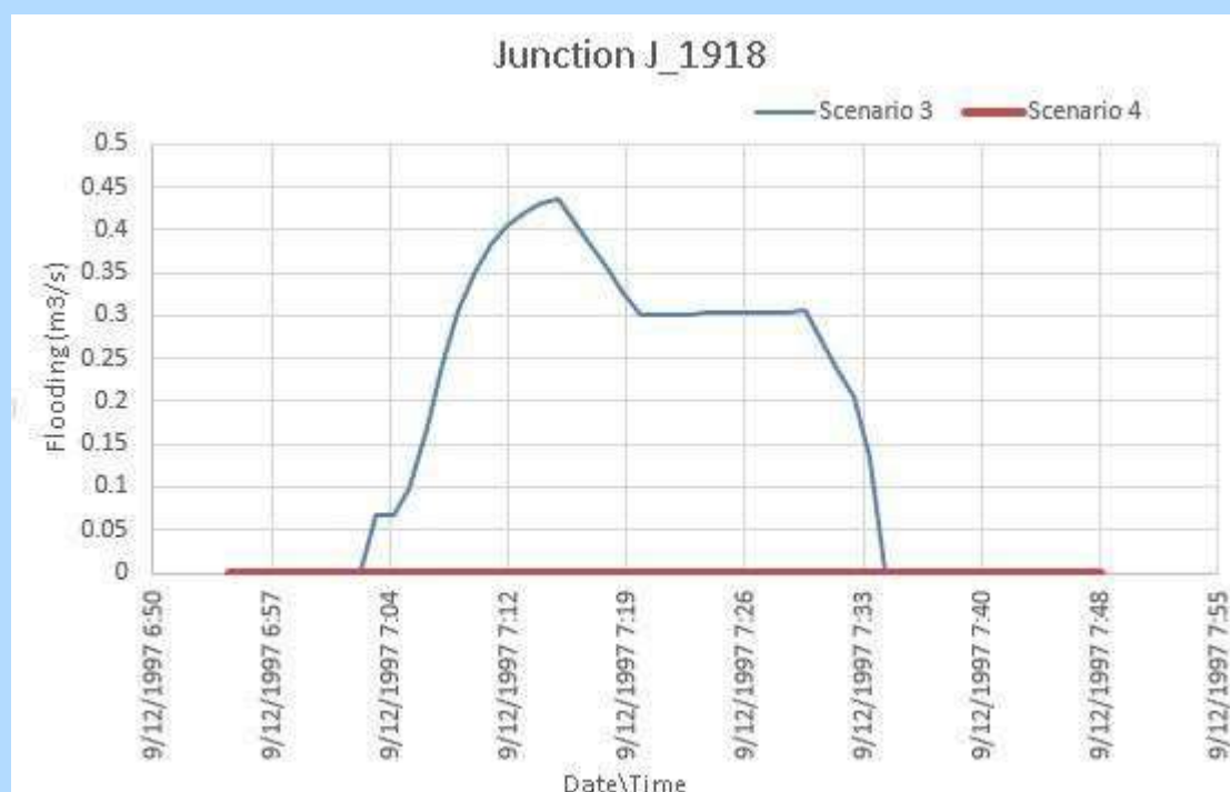
Figure 3.1-18: Comparison between the flood volume at a sample junction after simulation of scenario 3 and scenario 4
